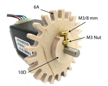
The cog 6A needs to be securely joined to the shaft of the stepper motor. Glue 10D to the cog and insert the M3 screw and nut as shown.
