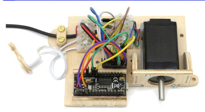
The motor is powered by a standard USB phone charger, this is not included because of differing plug standards. Cut off the plug at cable end and strip back to the red (plus) and black (minus) wires and screw into the screw terminal.
