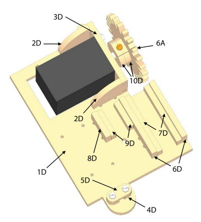
The motor and controllers are assembled on a separate board which when finished is simply screwed into the bottom of the clock base.
