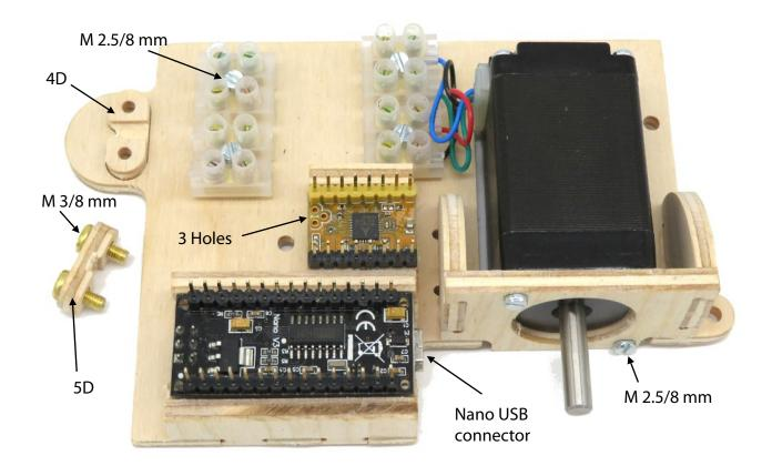
Glue 4D into the recess on the base 1D, when you have wired up the cable to the USB charger screw on 5D to clamp it.
